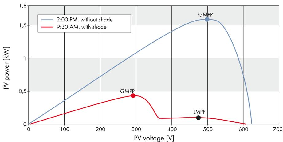
Fig. 1: Power-voltage diagram of the represented PV array at two different times of day (with and without partial shade). The curves show that there are two MPPs with different qualities when there is shade, with the power at the local MPP being significantly lower than that at the global MPP.
