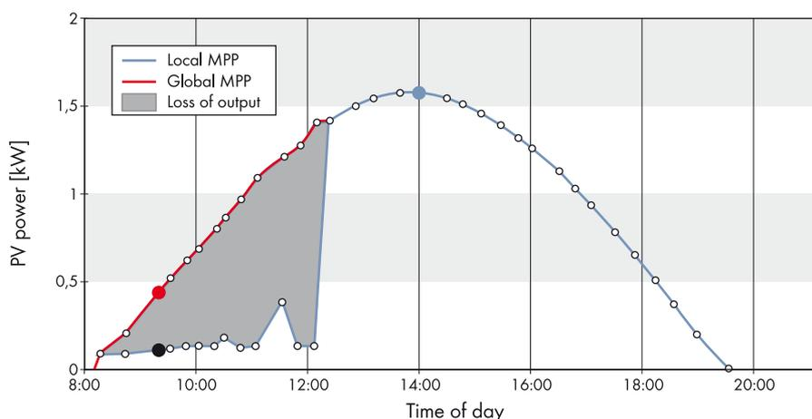
Fig. 2: Course of the global and local MPP power of a partial array of a PV system with morning shade. The gray area shows the loss of output that would be caused by setting the local MPP instead of the global MPP.
