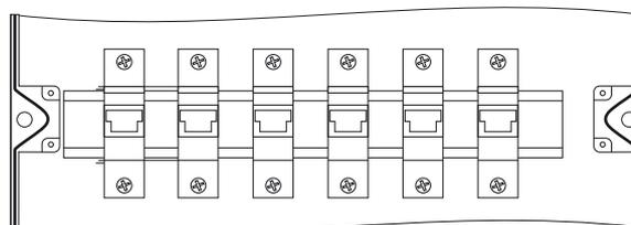
The deduction for heat impairment is designated as adding factor. This factor is specified in the technical data of the circuit breaker. With an arrangement of nine devices, for example, the adding factor can be 0.77. The circuit breaker with a nominal current of 50 A behaves as if its nominal current was  $0.77 \times 50 \text{ A} = 38.5 \text{ A}$ .
